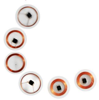
APK-ID clear tag comes in different shapes, sizes, frequency and protocol. These tags are ideal choice for embedding inside machines, plastic parts or wood. This tag is available in different frequencies (LF and HF) and protocols.
